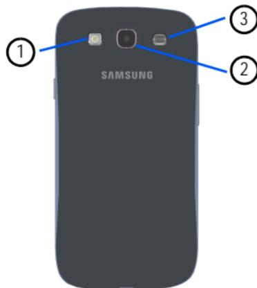
1. **Flash:** is used to provide adequate light when taking pictures in dark places.
