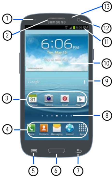
1. **Status light:** displays red when charging, green when fully charged, blue when powering up, and orange when a
