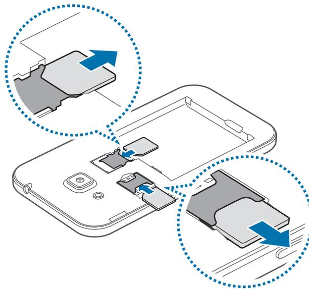
▶ **Single SIM models:** Press the SIM or USIM card with your finger, and then pull it out.
