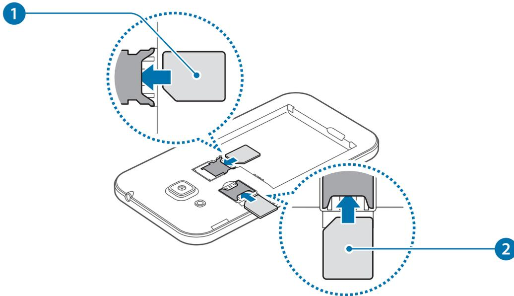
► **Single SIM models:** Insert the SIM or USIM card with the gold-coloured contacts facing downwards.
