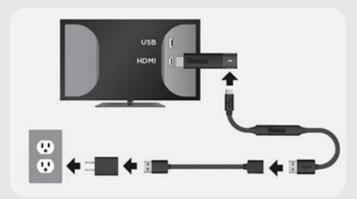
First, plug your Roku Streaming Stick into the HDMI port of your TV. Next, use the USB power cable, power extender cable, and power adaptor to connect your device to an outlet.
